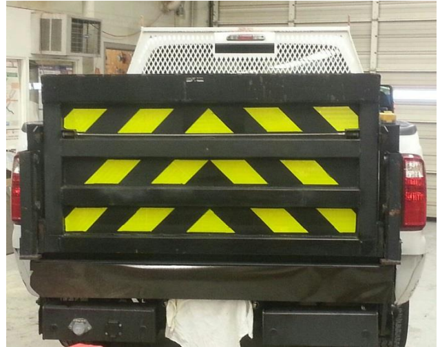
CHEVRON PATTERN ON LIFT GATE
